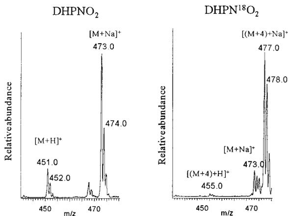
**Figure 1.** Mass spectrometry analysis of the DHPNO<sub>2</sub> and DHPN<sup>18</sup>O<sub>2</sub>.
