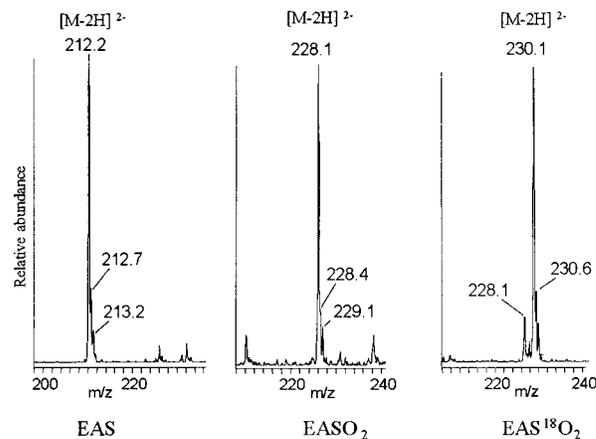
**Figure 2.** Mass spectrometry analysis of the EAS, EASO<sub>2</sub>, and EAS<sup>18</sup>O<sub>2</sub>.
